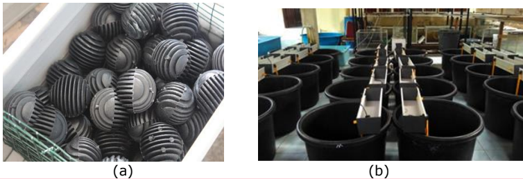
Figure 1. a. Bioball used as a filter substrate, b. The design of the Silver pompano aquaculture recirculation system.
