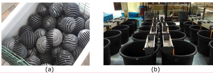
Figure 1. a. Bioball used as a filter substrate, b. The design of the Bawal Bintang aquaculture recirculation system.
